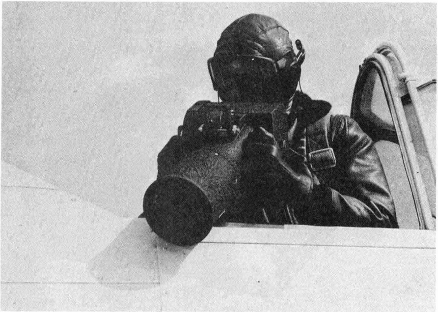
FIG. 2-2. Type CA-6a camera, 4-in. by 5-in. photographs, 15-in. focal length, used for hand-held oblique photography. (Photo from files of Gordon Enterprises.)
