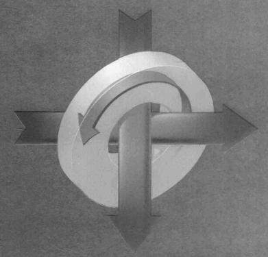
Splitting the current. Each of the wires threaded through the core above carries half the current needed to magnetize it. Alone, neither current would affect the core, but when the two currents join forces-or coincidethe core is magnetized according to a double application of the right-hand rule, in this case as a one. Reversing the current in both wires flips the magnetic field of the core, marking it as a zero.
