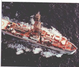
Figure 21.15 The JOIDES Resolution. This modern oceanographic research vessel drills for sample sediments beneath the ocean floor.
