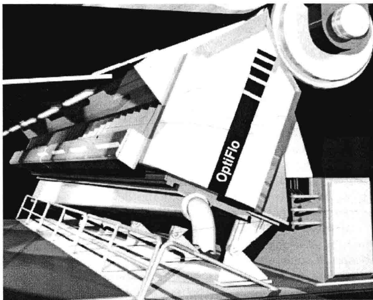
Fig. 2. The headbox of a paper machine.
