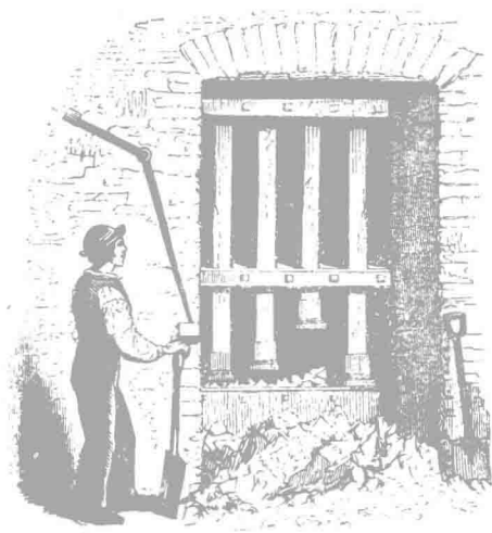
Fig. 1.1. Stamp Mill for crushing flints for the manufacture of Porcelain (Tomlinson: Illustrations of Useful Arts, Manufactures and Trades , 1867).
