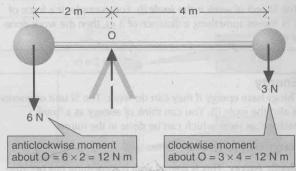
The dumb-bell is made up of smaller parts, each with its own weight. Together, these are equivalent to a single force, the total weight, acting through O. O is the *centre of gravity* of the dumb-bell.
