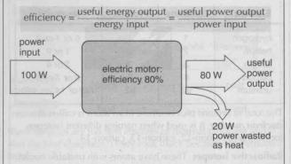
For example, if an electric motor's power input is 100 W, and its useful power output (mechanical) is 80 W, then its efficiency is 0.8. This can be expressed as 80%.
