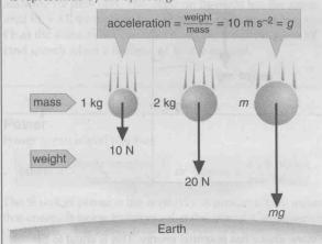
In the diagram above, all the masses are falling freely (gravity is the only force acting). From F = ma, it follows that all the masses have the same downward acceleration, g. This is the **acceleration of free fall**.
