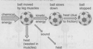
Whenever there is an energy change, work is done – although this may not always be obvious. For example, when a car's brakes are applied, the car slows down and the brakes heat up, so kinetic energy is being changed into internal energy. Work is done because tiny forces are making the particles of the brake materials move faster.
