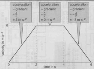
On the velocity-time graph above, you can work out the acceleration over each section by finding the *gradient* of the line. The gradient is calculated like this:
