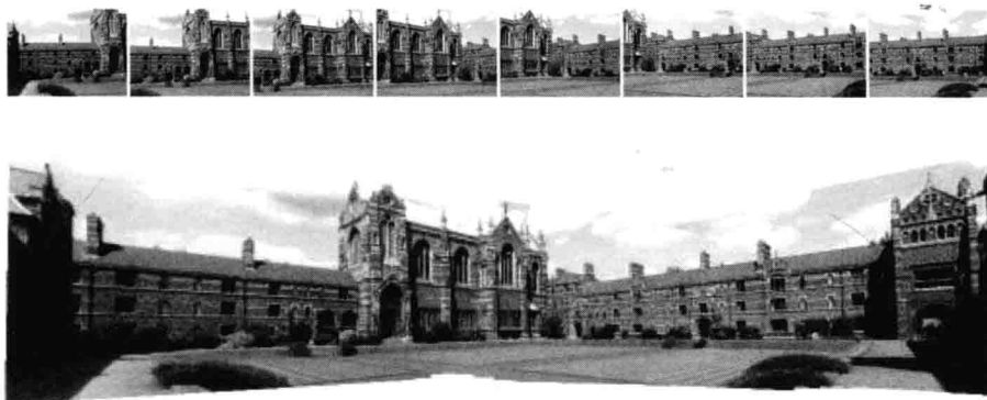
Figure 1.3: (Top) 8 frames from a sequence of 25 captured by a hand-held video camera. (Bottom) All 25 frames are combined by image mosaicing. The field of view is greatly increased.
