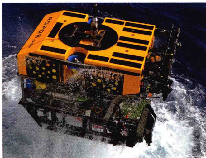
Figure P.3 The remotely operated vehicle ROPOS surfaces in the Pacific Ocean after a dive to 2500 m (8200 ft) on the Juan de Fuca Ridge. Robotic vehicles similar to this one explore the depths using high-bandwidth fiber-optic cables, thereby permitting detailed exploration of over 98% of the global seafloor down to 6500 m (21,320 ft) depth.
