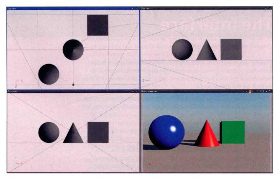
In this figure, you see in the top view that these figures are placed so the sphere comes before the cone, which comes before the cube, and that they are also displaced along the X axis. However, the objects appear to be in perfect alignment in the front and side views because of their orthogonal view. It is in the camera view where you see the effects of perspective, showing not only smaller shapes in the distance but also an appearance of being off center in the camera's field.
