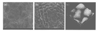
Figure 1.3 Environment SEM (ESEM) images (a & b) show its lower side is made of many cells, and every cell consists of numerous tabular and slightly convex papillae with 30-50 µm in length and 10-30 µm in width. (c) Atomic force microscope (AFM) image further shows the tabular papillae are covered with nanogrooves structure with a size of 200-500 nm and the height of single papilla is around 4 µm.
