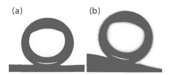
Figure 1.4 (a) Lower side of lotus leaf shows superoleophobicity with oil contact angle (OCA) of  $155.0 \pm 1.5^{\circ}$  for 1, 2-dichloroethane. (b) When the tilt angle reaches about  $12.1 \pm 2.4^{\circ}$ , the oil droplet easily rolls off from its lower side.
