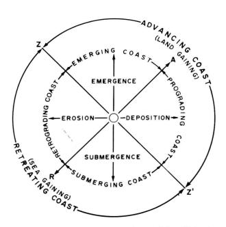
Fig. 1 Analysis of coastline change (after Valentin, 1952). Z–Z' indicates a stable coastline, where erosion has been offset by emergence, or deposition by submergence, or where no changes have taken place (O). It is necessary to specify a time scale over which changes have taken place before using this scheme, for many coastlines have shown alternations of advance and retreat during the past century
