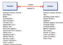
FIGURE E13.1 Unnormalized entity-relationship diagram for the computer system. The many-to-many relationship will have to be defined as an associative entity.
