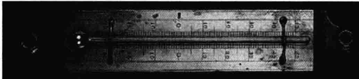
Celsius thermometer (attached to a barometer) made by J. G. Hasselström, Stockholm, late eighteenth century.
