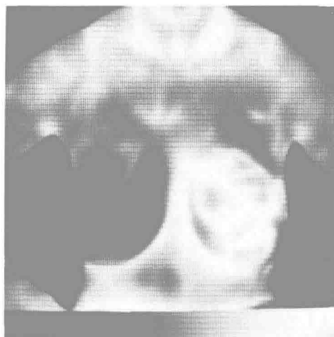
Figure 1.1. A typical monochromatic thermogram. The calibration scale at the bottom runs from cold on the left to hot on the right. In this example white areas are the hottest and black areas are the coldest.
