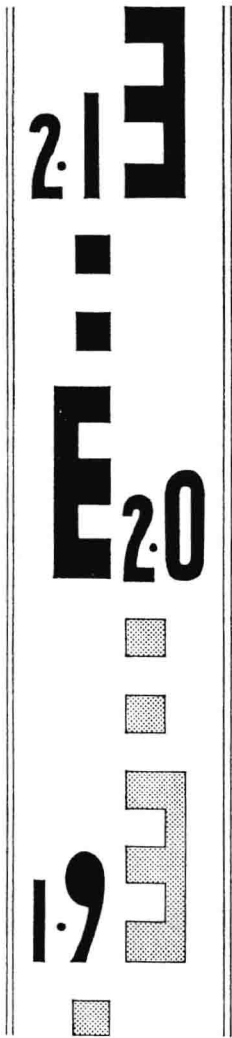
1.17 Levelling staff marked in 10 mm increments
