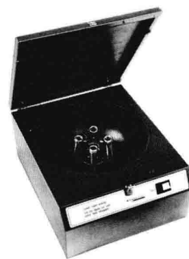
Figure 3 A centrifuge is used to separate the solid from the liquid in a suspension. When the centrifuge is switched on, it spins at high speed; the buckets containing the test tubes swing out, and the solid is flung to the bottom of the test tube.
