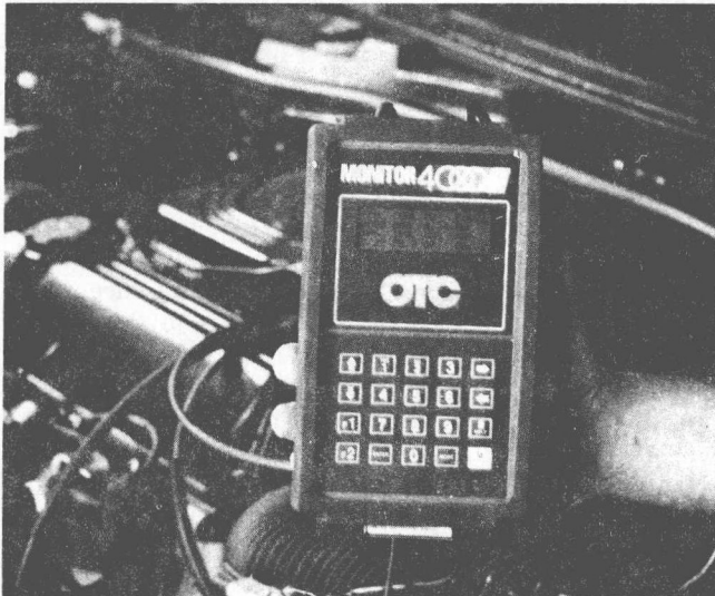
Fig. 1-16. Checking for diagnostic codes with a diagnostic tester. (OTC Tool and Equipment Division of SPX Corporation)
