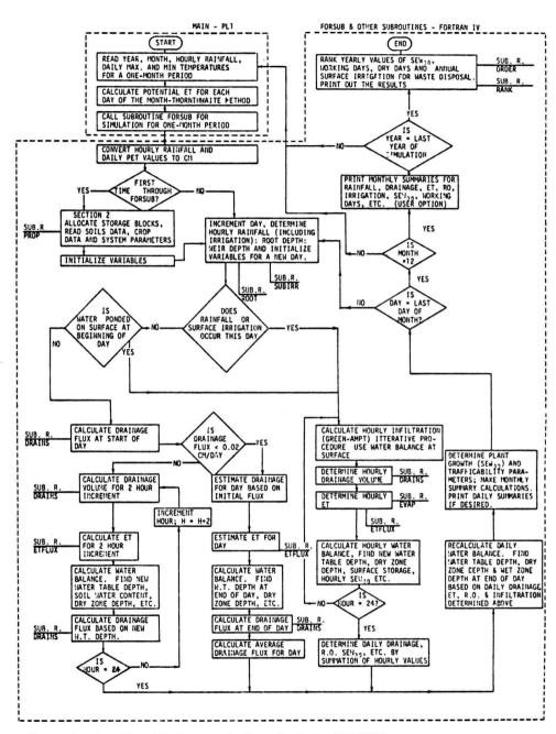
Figure 2. An abbreviated general flow chart for DRAINMOD.
