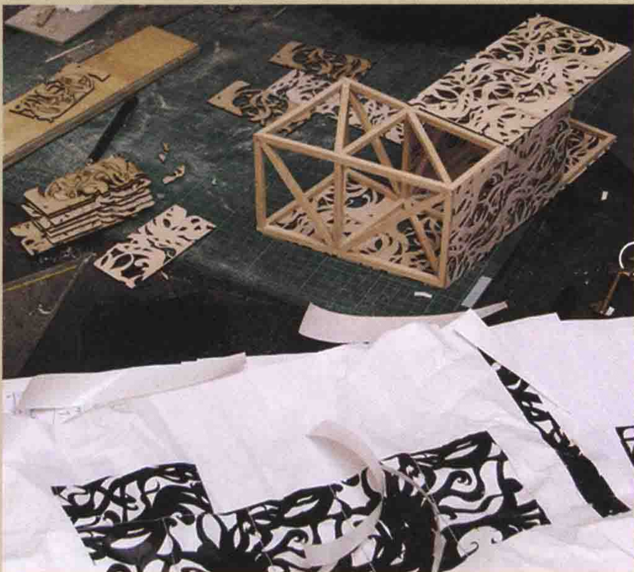
1:20 model of a temporary pavilion by 6a architects in the process of being made. The intricate pattern directly replicates that of the final intervention and uses the same process of manufacture, albeit on a smaller scale.
