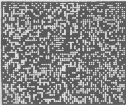
FIG. 19-8 Random arrangement of black and white particles. [Lacey, Trans. Inst. Chem. Eng. (London), 21, 52 (1943).]
