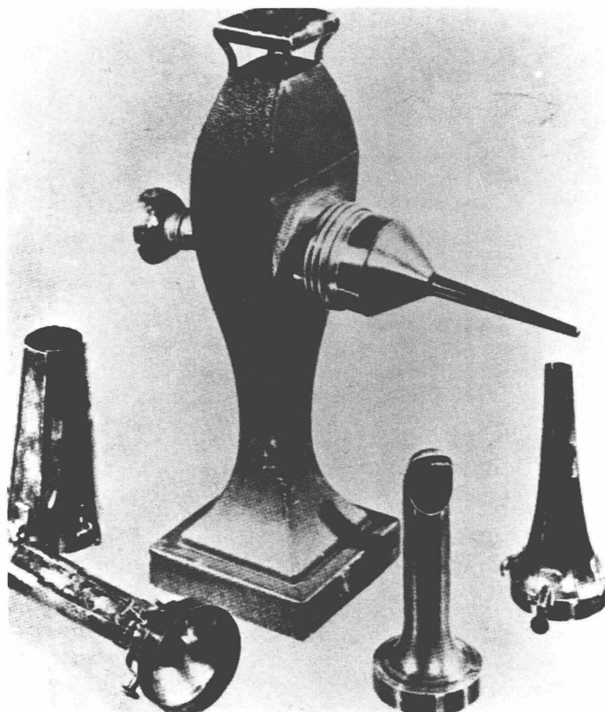
FIG. 1-1 Instruments described by Bozzini in 1807 treatise. 5 Vase-shaped apparatus was 37 cm high, 3.2 cm in depth, and 8 cm in width.
