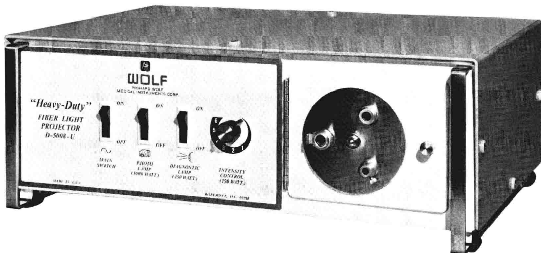
Fig. 1-11. Photographic fiber light projector with two alternating light sources.
