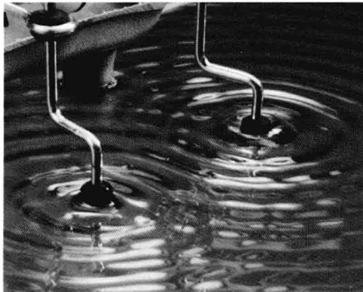
Interference of water waves produced in a ripple tank. The sources of the waves are two objects that vibrate perpendicularly to the surface of the tank. (Courtesy of Central Scientific CO.)
