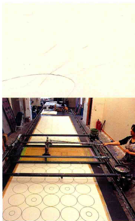
At Double Helix's studio in Glasgow, a 10m print table incorporates a 'carriage', allowing large-scale printing to be carried out by one person.
