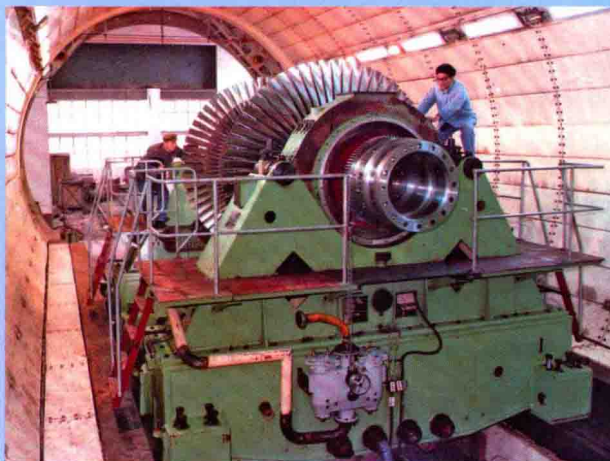
China's first self-developed 200t high-speed balancing equipment
