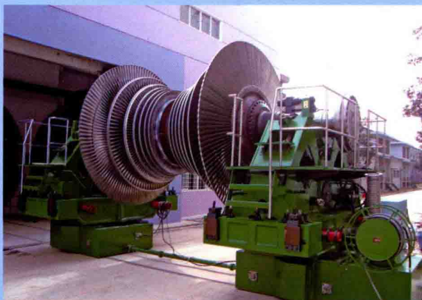
A turbine Rotor waiting for high-speed balancing
