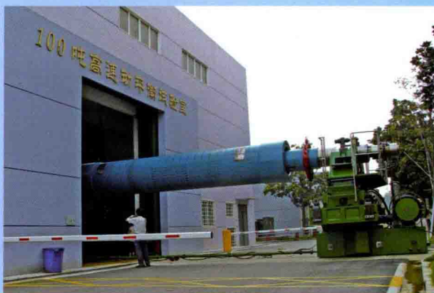
100t high-speed balancing and overspeed test chamber
