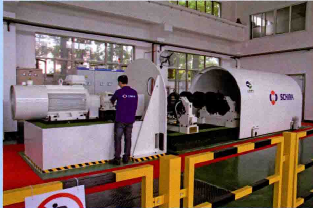
4.5t high-speed balancing and overspeed test chamber
