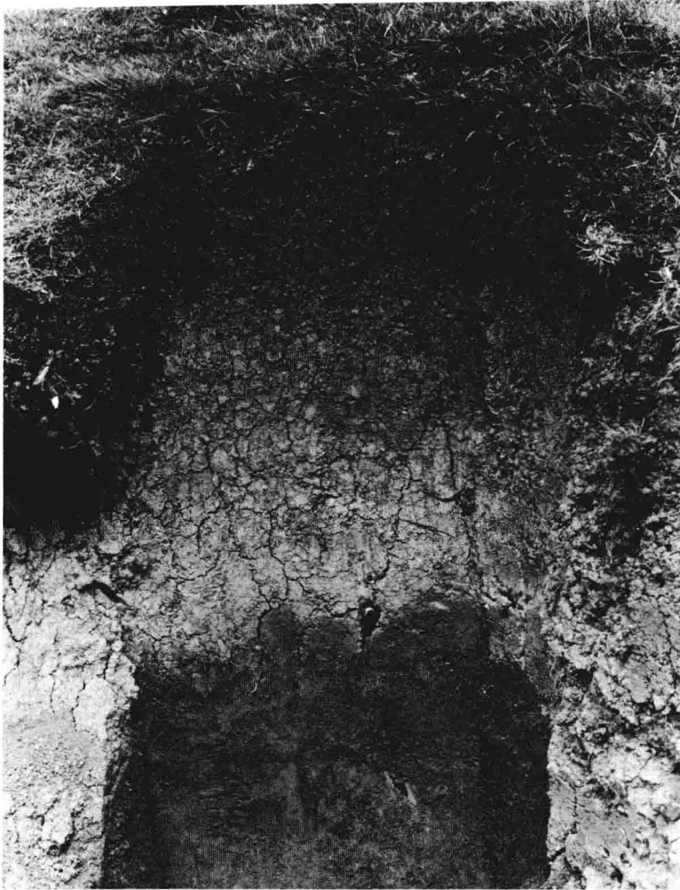
2.2 A soil with high kaolinite content formed on a sandstone. The presence of clay minerals is indicated by the shrinkage from drying of the upper part of the profile. The lower part of the profile is still moist.
