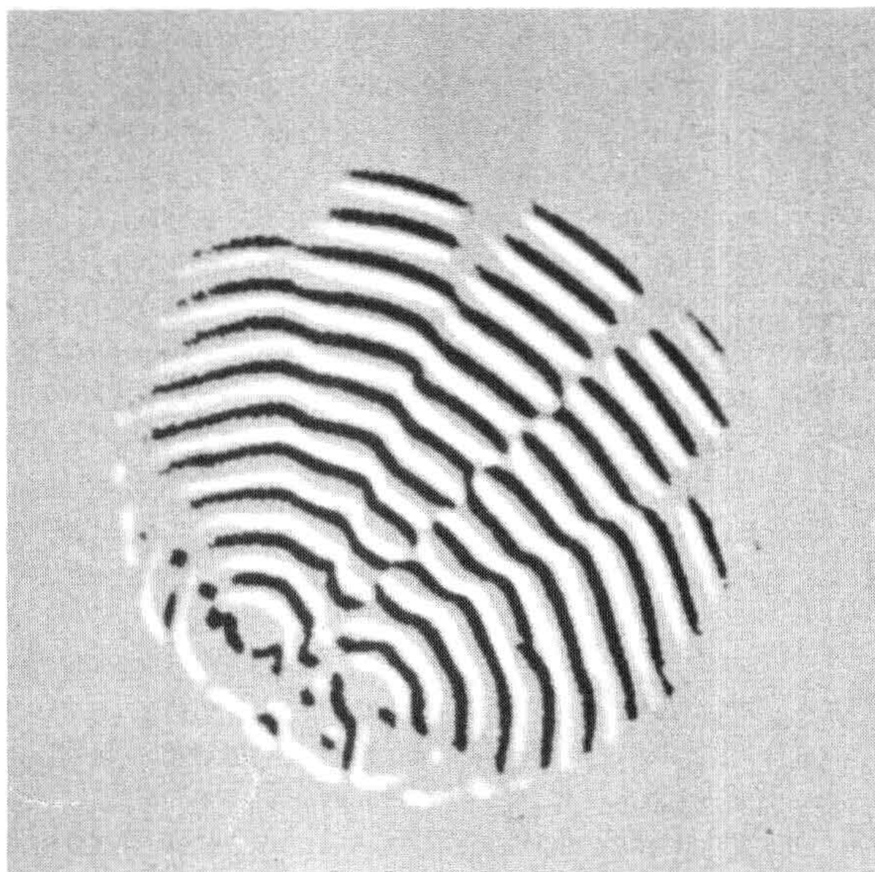
Fig. 1.4 Photograph of the interference pattern produced by two vibrating sources in water.
