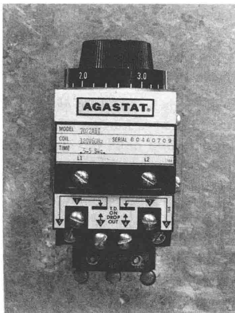
Pneumatic off-delay timer. A microswitch has been added to the bottom to supply instantaneous contacts for the timer.
