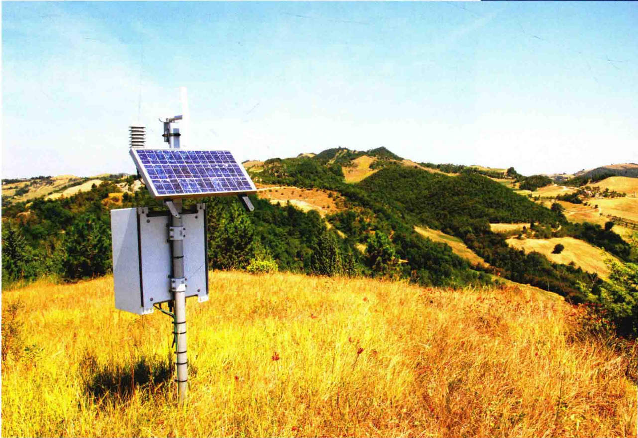
Automatic weather station in the Apennine Hills near Madigliana, Romagna, Italy.
