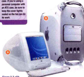
Figure 2.3 a&b (a) The Apple iMac's system unit sits on the desktop and also contains the computer's display. (b) The Macintosh G4 uses a tower case that sits on the floor next to the desk.
