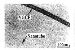
Fig. 1.1: High resolution TEM micrograph showing carbon nanotubes with diameters less than 10 nm [14-17].
