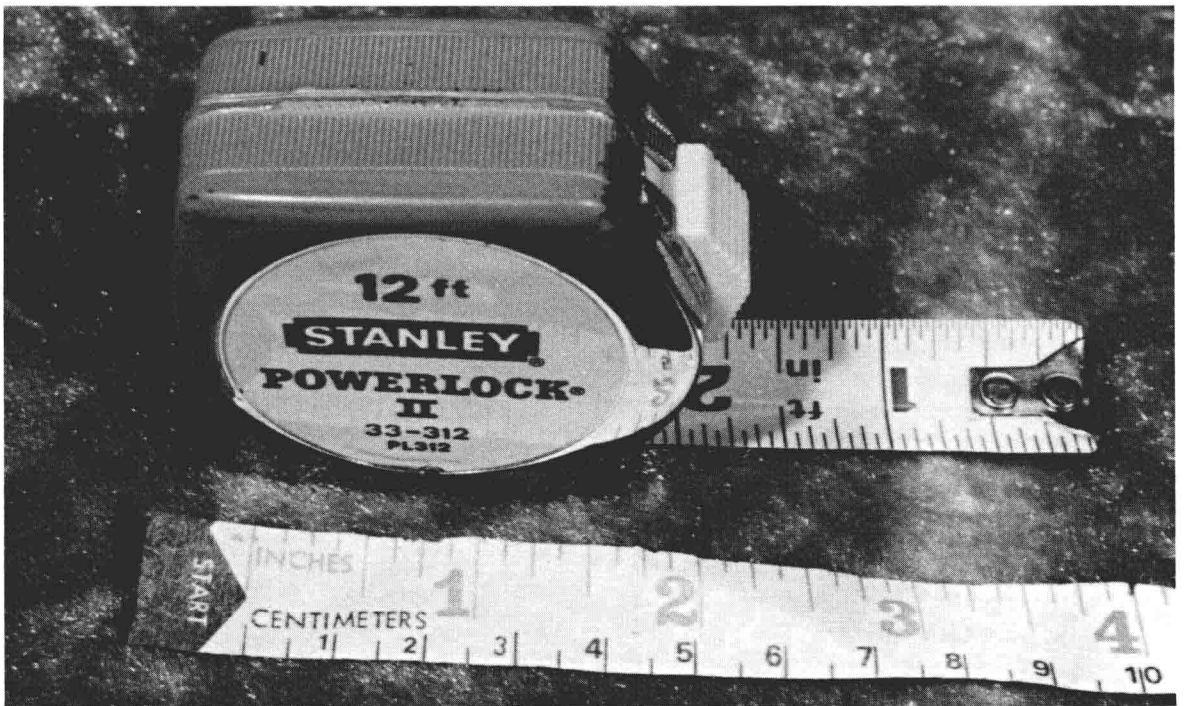
Fig. 2-3. Flexible measuring tapes: top-steel rule, bottom-cloth tape.
