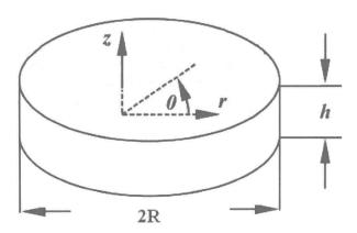
Fig. 1. The geometrical configuration of the piezoelectric ceramic disk.
