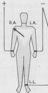
FIGURE 13. Electrical connections of standard lead aV_R .
