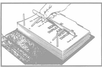
☐ When all the material has been returned to the retainer bar, replace the lifter bar. Close the volume by bringing the cover of the binder into place and pushing it firmly on to the retainer bar. Make sure that the binder is properly closed before replacing it on the shelf.
