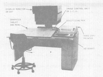
Components of a typical workstation.
