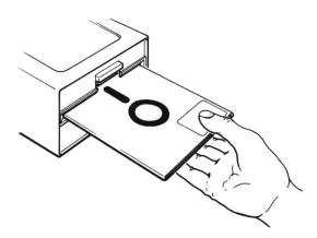
Gently push the disk entirely into the drive. *Do not bend!* Pushing too hard will surely damage it. Close the door by pressing it down all the way. The door lowers and raises the head from the disk, just like a phonograph needle—so slowly and gently are the watchwords.
