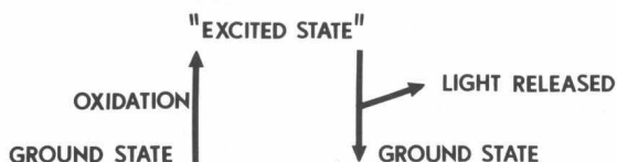
FIGURE 2. Schematic diagram depicting the production of light from certain molecules in the excited state. The same change in energy levels occurs as in Figure 1 with the exception that upon return to ground state light is released. The initial change from ground state to an excited state could be accompanied by an oxidation of the initial molecule in ground state.
