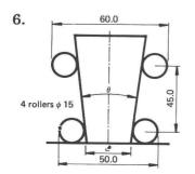
Dimensions over two sets of identical rollers at different heights are shown. Calculate
