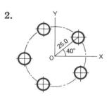
Five holes are equally spaced on a pitch circle of 50.0 mm diameter. Compile a table showing the five co-ordinate hole centres.
