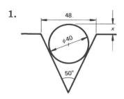
A test plug,  $40 \, \text{mm}$  in diameter, rests in a  $50^{\circ}$  vee-groove. Calculate x, the distance the top of the plug protrudes above the top of the groove.
