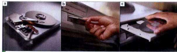
FIGURE 1.10 The most common storage devices are (a) a hard disk drive, (b) a floppy disk drive, and (c) a CD-ROM or DVD-ROM drive.
