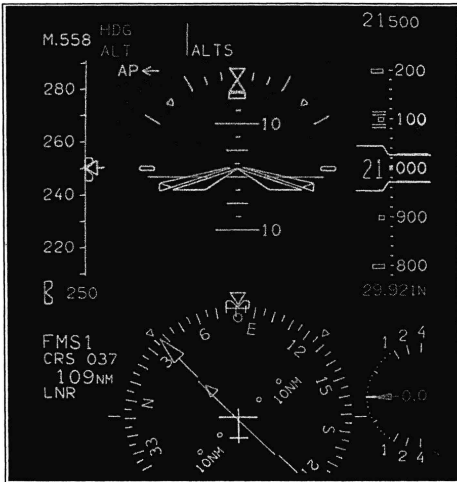
Figure P-1. Rockwell Collins Proline 4 Primary Flight Display. (Courtesy Rockwell Collins Avionics)
