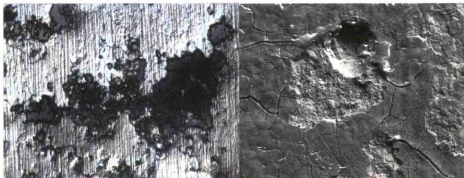
Fig. 3. SEM images showing the pitting corrosion for the aluminium
