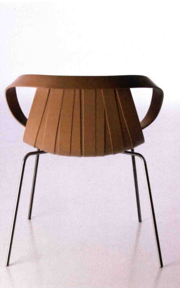
Above: Impossible Wood , Doshi Levien for Moroso, 2011. This armchair is injection moulded using a thermoplastic composite of 80 per cent wood fibre and 20 per cent polypropylene.
