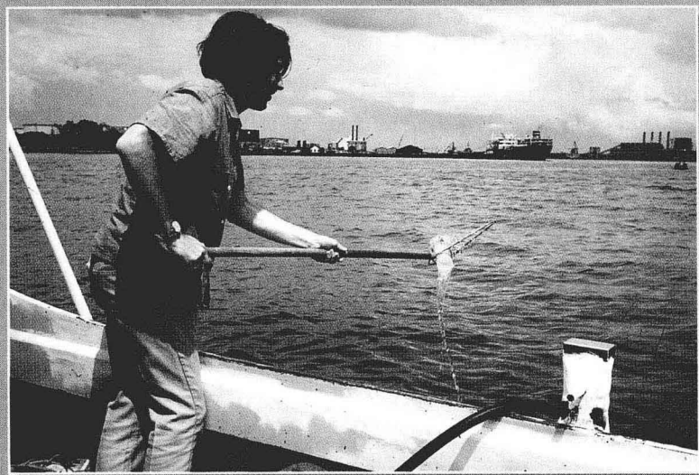
Collecting water samples in Prince William Sound, Alaska, to study microbial degradation of oil.
