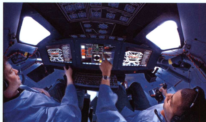
Orion's instrument panel uses flat screen displays to simplify the layout. <
