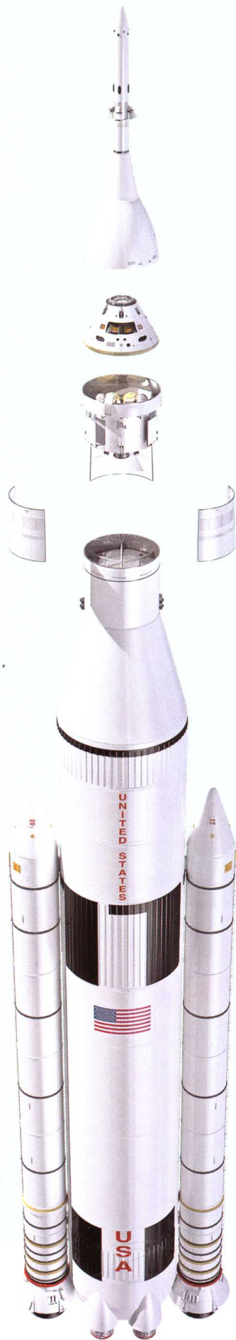
The Space Launch System (SLS) will be assisted at lift-off by solid rocket boosters developed from space shuttle technology. ◀
