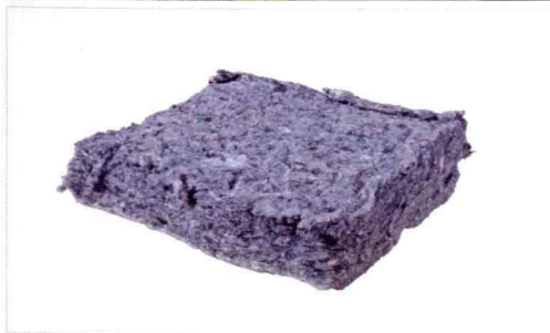
Above: California Academy of Sciences, San Francisco, California, USA, 2008. Photo by Taisuke Inatsugu / Shinken-chiku-sha. Below: Recycled denim insulation. Photo courtesy of RPBW, Stefano Goldberg - Publifoto.
