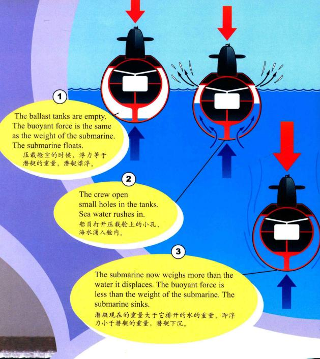
To dive, the crew fills the ballast tanks with water. The density of the submarine is now greater. The submarine is heavier than the water it **displaces**. The submarine sinks.
