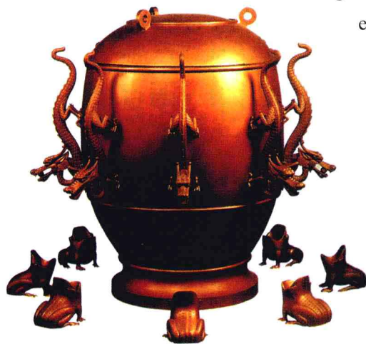
Earthquake Sensor invented by Zhang Heng, Han Dynasty.
