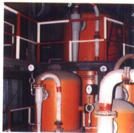
△VOD精鍊爐用蒸汽噴射真空泵 Steam-Ejection Vacuum Pump of the VOD Refining Furnace
