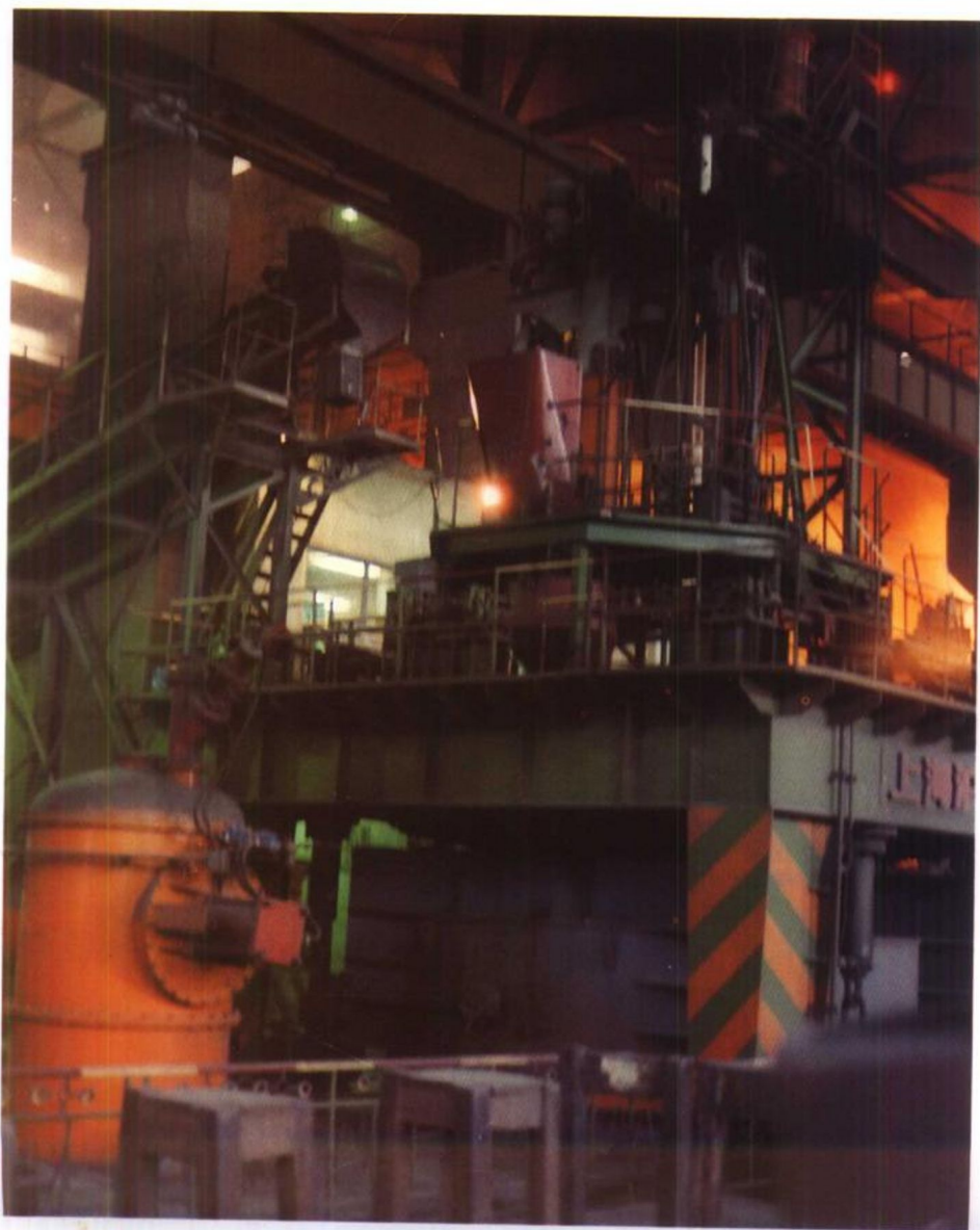
△VOD精鍊爐用蒸汽噴射真空泵 Steam-Ejection Vacuum Pump of the VOD Refining Furnace
