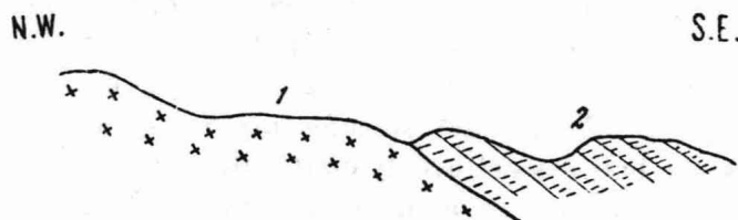
Fig 1. An ideal section across the Contact Metamorphic Zone of Tien-o-pautan to show the relation between the pure contact silicates with the garnetiferous magnetite. Here the quartz diorite is not exposed to view.
